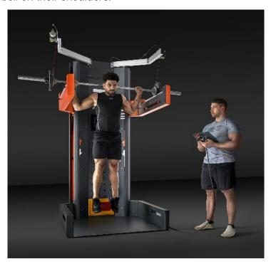
Without the support of the lifter, the additional weight would be limited by the fact that the athlete must absorb this weight upon landing after performing the jump. The lifter supports athletes in this exercise by following the bar upwards with its arms during the jump and intercepting it at the highest point. This means that the athlete does not have to absorb the weight themselves upon landing.
